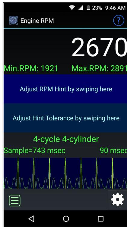
probably set wrong. You should adjust the RPM range, as described later, until the yellow lines do line up with the peaks in the graph.
